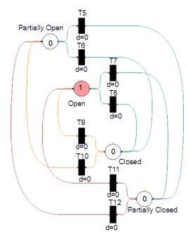
Figure 5. Operational states of the valve
