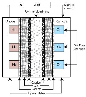
Figure 1. Structure of a PEM fuel cell.
