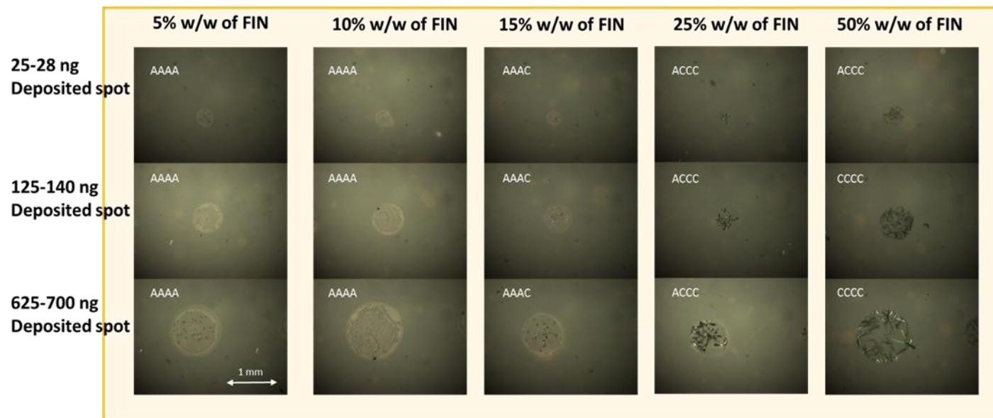
**Figure 3. Example of an array section, all the POM pictures are reported with the cross polarized filters in place. Pictures of all Finasteride-PVPVA spots at all the different ratios are depicted after 7 days from the solvent evaporation. As shown in each row there is the same amount of printed materials (25-28ng top row, 125-140ng center and 625-700ng bottom row) and in each column there are spots containing the same drug/polymer ratio.**
