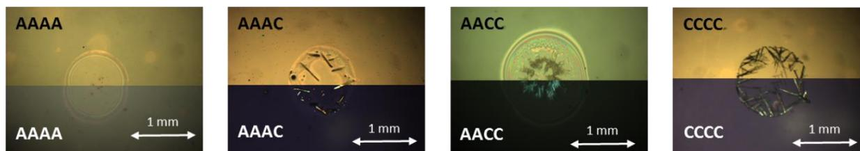
**Figure2.** Examples of different API recrystallization profiles are presented. All the pictures are reported both without (top part) and with (bottom part) a polarized filter. (i) AAAA stands for entirely amorphous, (ii) AAAC, mainly amorphous, (iii) AACC, mainly crystalline and (iv) CCCC, entirely crystalline.
