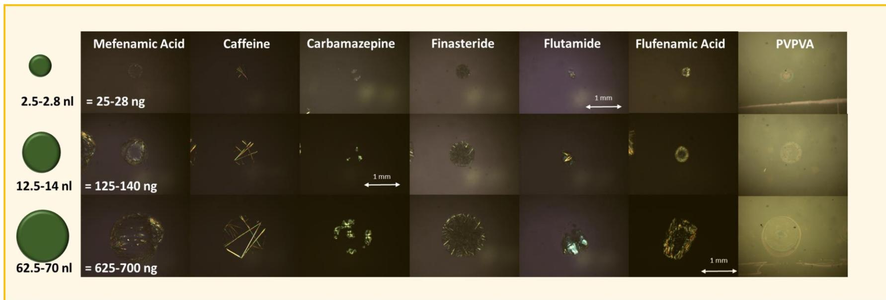
**Figure 2SI.** Pure drugs and PVPVA microarray depicted by POM with the polarizing filters on. From the top line: spots produced by depositing a volume solution between 2.5-2.8 nl (25-28 ng). Middle line: spots printed using 12.5-14 nl (125-140 ng). Bottom line: spots printed with a volume ranging 62.5-70 nl (625-700 ng). All the drugs but not the amorphous polymer show a characteristic birefringent pattern. In fact, PVPVA is barely visible with the polarizing filters on.
