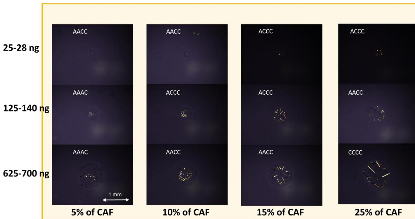
Figure 4SI. Drug-PVPVA spot array POM pictures, varying both printed amount (number of droplets) and drug polymer ratio.
