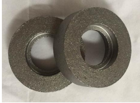
Fig. 3 Specimen of ring with an inner boss
