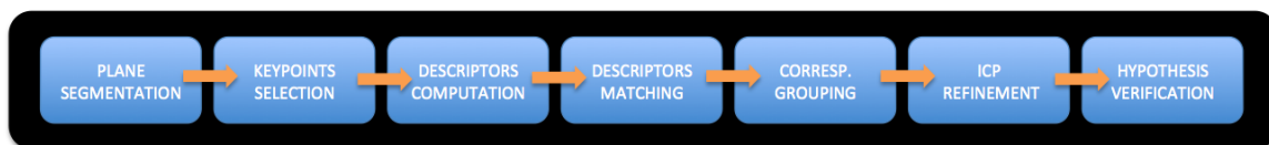
Fig.3. The recognition and pose estimation algorithm pipeline.
