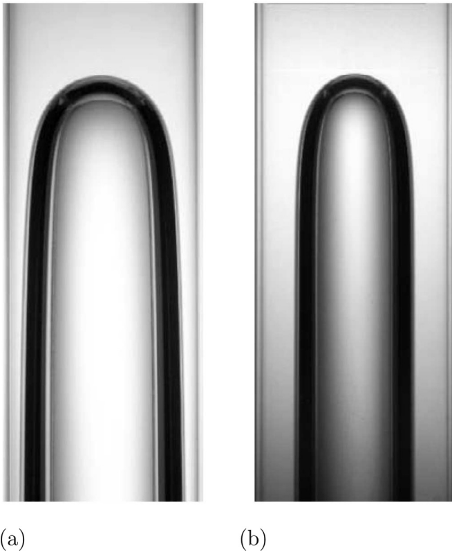
Fig. 1. Examples of an air Taylor bubble rising through (a) water and (b) silicone oil [7].
