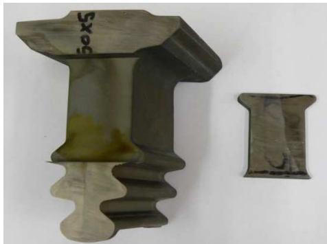
Figure 8: Piece of root extracted along the main direction of the blade.
