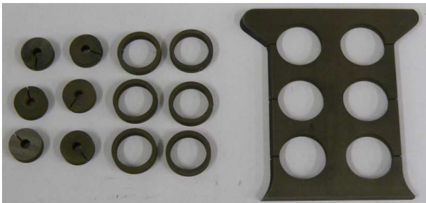
Figure 9: Ring specimens and remains from EDM operations.
