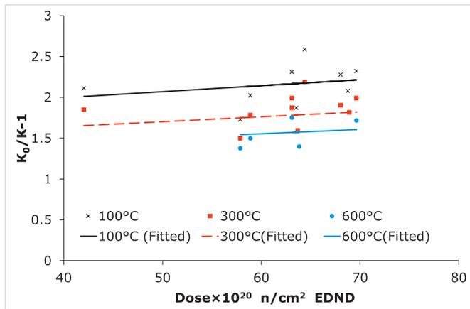
**Fig. 2.** Thermal resistivity variation with fast neutron dose as a function of dose and temperature as fitted by the proposed formula compared to experimental results from [12] (for 100 °C, 300 °C and 600 °C).
