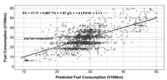
Scatter plot for Predicted Fuel Consumption and Real Measurements
