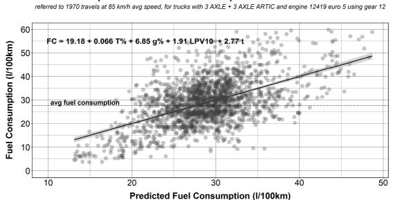
Scatter plot for Predicted Fuel Consumption and Real Measurements
