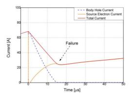
Figure 7. Current components during avalanche breakdown.
