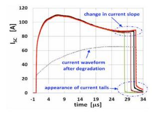
Figure 11. SC current waveforms for  $V_{\rm DS}\,{=}\,400$  V,  $T_{CASE}\,{=}\,90$  °C and varying pulse width.
