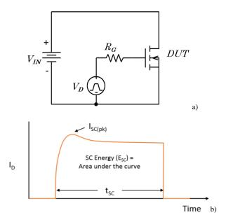
Figure 10. SC test circuit schematic, a), and representative current waveform, b).
