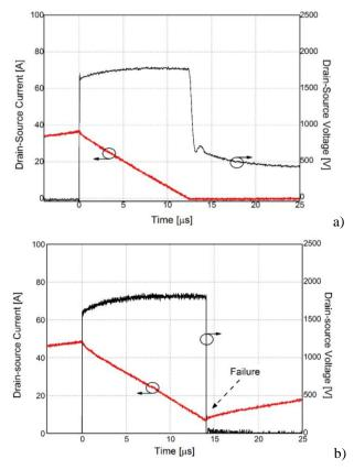
Figure 3. In a), safe UIS and avalance breakdown event; in b), destructive event.
