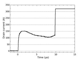
Figure 12. SC current waveforms for  $V_{DS} = 400$  V,  $T_{CASE} = 90$  °C.
