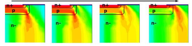
Figure 8. Progressive re-distribution of the curent density within the device structure during the avalanche event, encompassing the time before and after failure.
