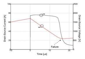
Figure 5. Simulated current and voltage waveforms for a destructive UIS and avalance breakdown event. Failure is defined as the moment where the voltage collapse takes place.
