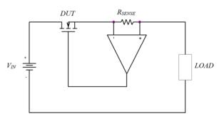
Figure 16. Test circuit schematic for device use as current limiter and regulator.
