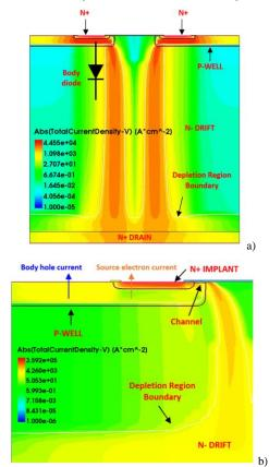
Figure 6. Current density distribution during avalanche breakdown: in a), far away from the time of failure; in b), just after filure.
