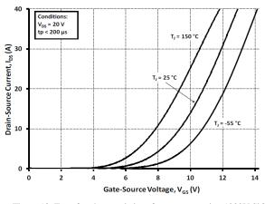
Figure 18. Transfer-characteristics of a new generation 1200V SiC MOSFET as per data-sheet information [3].
