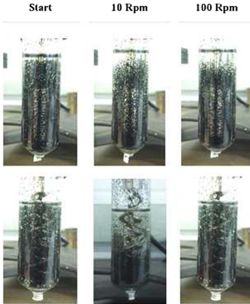
**Fig. 8.** Images of the distribution of particles in the viscometer using the f500 fluid for the SC4-27 spindle (top) and DHI (bottom) at the start of the test and after 10 minutes for various rotational speeds.
