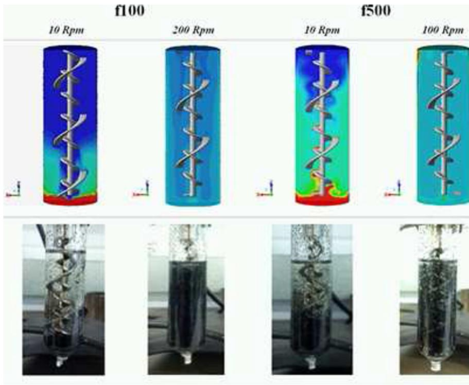
**Fig. 15.** Volume fractions from the CFD model (top) and experimental images (bottom) for the DHL. The volume fractions range from 0 (blue) to 0.08 (red). (For interpretation of the references to colour in this figure legend, the reader is referred to the web version of this article.)
