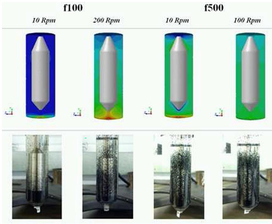
**Fig. 14.** Volume fractions from the CFD model (top) and experimental images (bottom) for the SC4-27 spindle. The volume fractions range from 0 (blue) to 0.08 (red). (For interpretation of the references to colour in this figure legend, the reader is referred to the web version of this article.)
