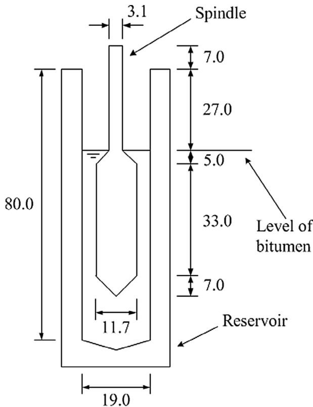
Fig. 4. A schematic of the Brookfield SC4-27 spindle.
