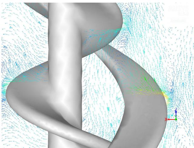
**Fig. 13.** A close-up of the inner and outer helices of the DHI impeller, showing the flow vectors on the plane  $y = 0$ . Vectors are the same length and the velocity magnitude is indicated by the color (blue is zero, red is  $0.061 \text{ m s}^{-1}$ ). (For interpretation of the references to colour in this figure legend, the reader is referred to the web version of this article.)
