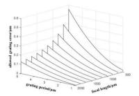
Figure 2: Allowed error in the grating period for the maximum central shift of 5  $\mu$ m, assuming wavelength  $\lambda = 0.5 \mu$ m
