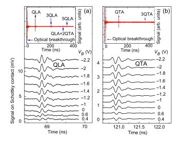
FIG. 2. Phonon-induced signals measured at pump fluence  $W = 4 \text{ mJ cm}^{-2}$  for various bias voltages  $V_B$  for (a) QLA and (b) QTA phonons. (Insets) QLA and QTA signals measured in a full temporal range.
