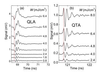
FIG. 3. Phonon-induced signals measured at zero bias,  $V_B = 0$  V, at various pump fluences for (a) QLA and (b) QTA phonons. Vertical dotted lines show the first-peak temporal shift to earlier times with the increase of *W* for QLA, and the absence of the shift for QTA phonons.
