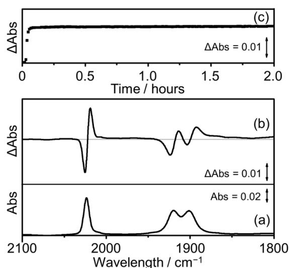
**Figure 5.** (a) FTIR ground state spectrum of  $[\text{ReCl}(\text{CO})_3(\text{dppz}-(\text{CH}_3)_2)]$  (0.5 mM) in a solution of  $\text{NEt}_3$  (1 M) and  $\text{CH}_3\text{CN}$ . (b) FTIR difference spectrum taken 0.5 hr after continuous photolysis at 420 nm. (c) Steady state photolysis kinetic trace for the formation of  $[\text{ReCl}(\text{CO})_3(\text{dppz}-(\text{CH}_3)_2)]^-$  recorded at  $2019 \text{ cm}^{-1}$ .
