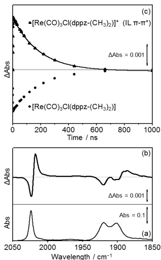
**Figure 2.** FTIR and ns-TRIR spectra of  $[\text{ReCl}(\text{CO})_3(\text{dppz}-(\text{CH}_3)_2)]$  (0.5 mM) in  $\text{CH}_3\text{CN}$ . (a) FTIR ground state spectrum. (b) ns-TRIR difference spectra taken 1 ns after excitation. (c) ns-TRIR single point kinetic traces for the decay of  $[\text{ReCl}(\text{CO})_3(\text{dppz}-(\text{CH}_3)_2)]^*$
