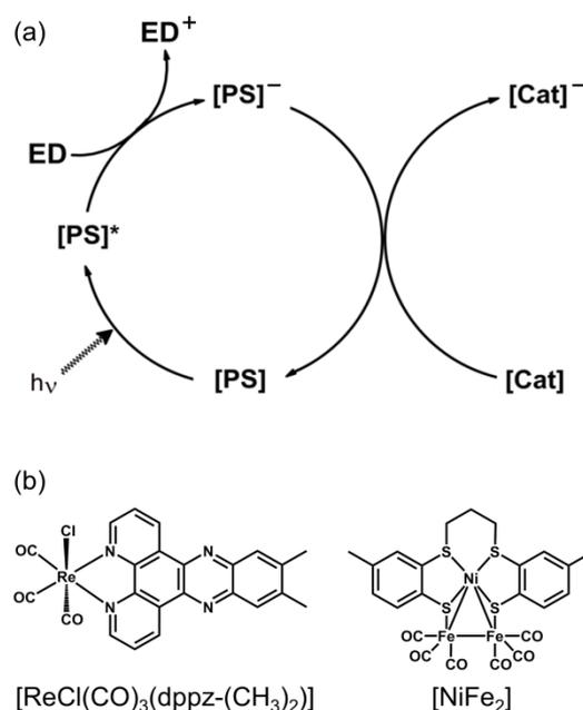
**Scheme 1.** (a) Simplified schematic of the one-electron reduction of a catalyst ([Cat]) by a photosensitiser ([PS]) proceeding *via* the reductive quenching of [PS]\* by an electron donor ([ED]). (b) Structures of  $[\text{ReCl}(\text{CO})_3(\text{dppz}-(\text{CH}_3)_2)]$  and  $[\text{NiFe}_2]$ .
