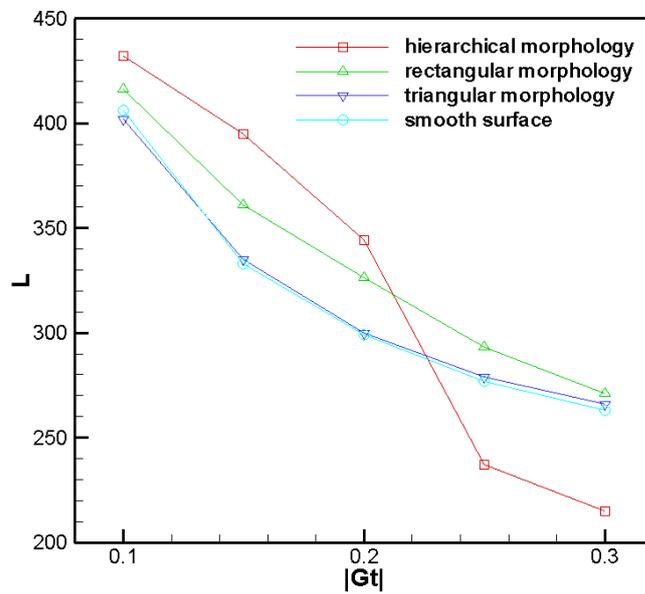
Fig. 15. Flow length in channels with different morphology
