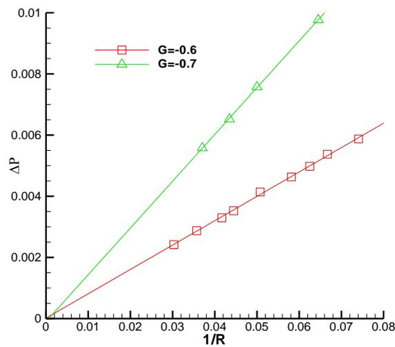
Fig. 6. The pressure difference as a function of its curvature with different fluid-fluid interaction strength
