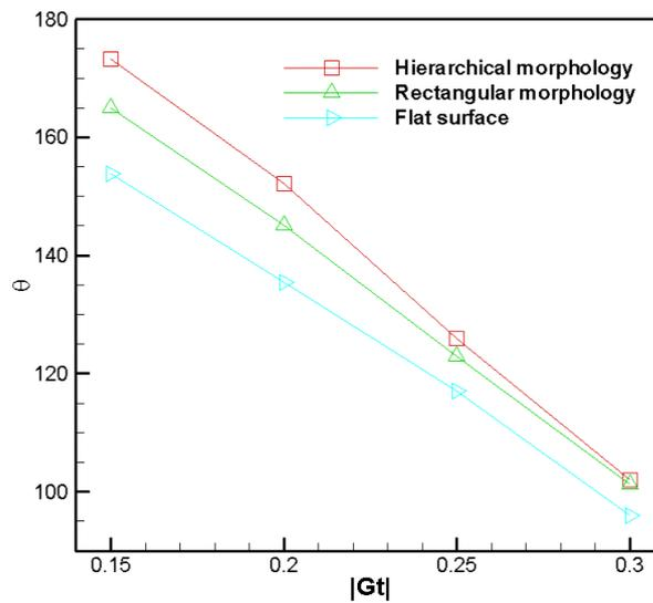
Fig. 9. Contact angles on different surfaces with different morphology
