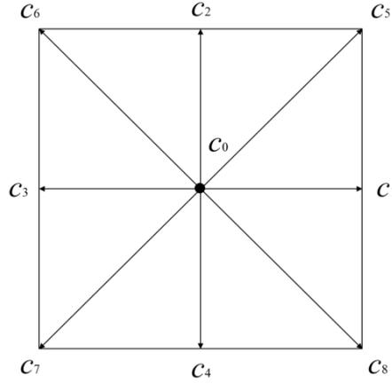
Fig. 1. Typical two dimensional lattice Boltzmann model (D2Q9)
