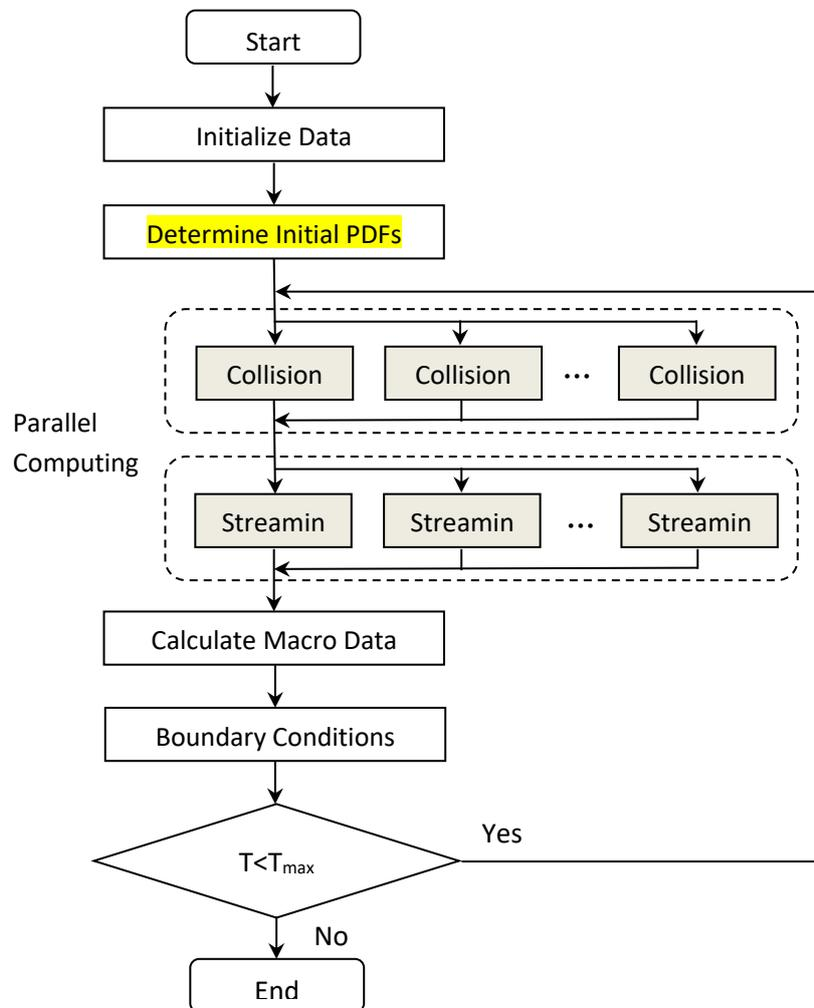
Fig. 3. Flowchart of the parallel LBM model
