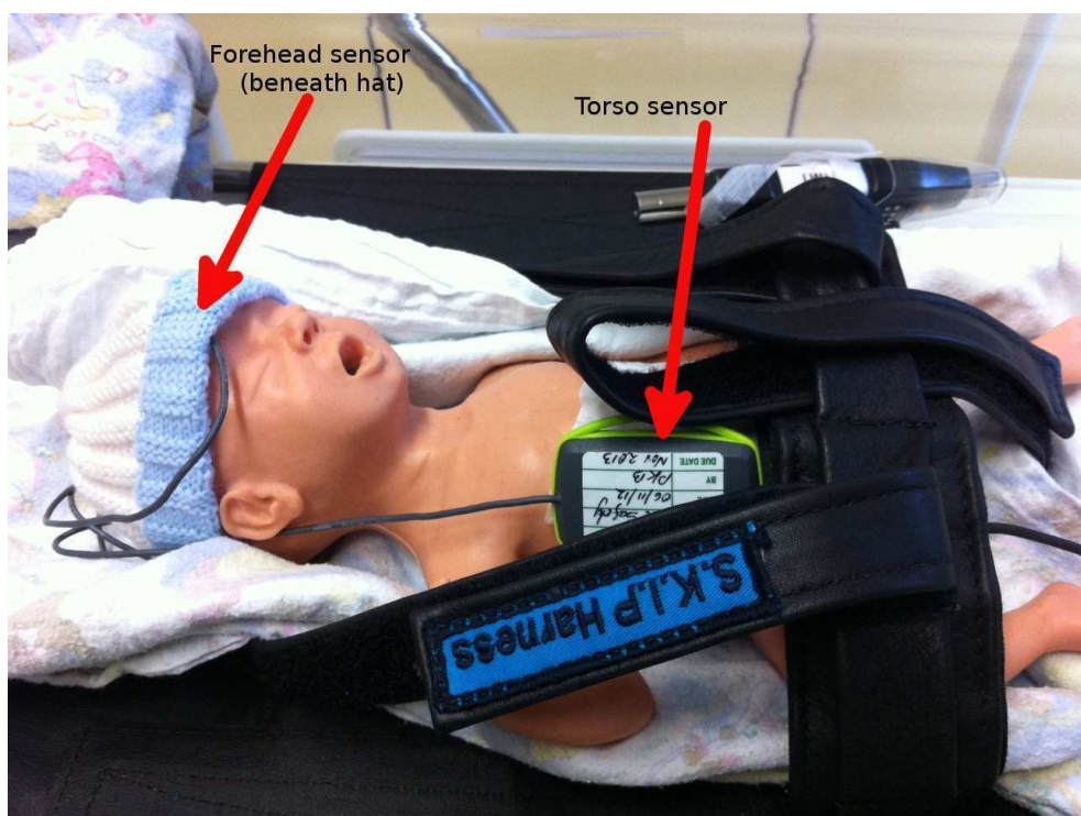
Figure 2. Labeled image of the sensors installed on a neonatal manikin.
