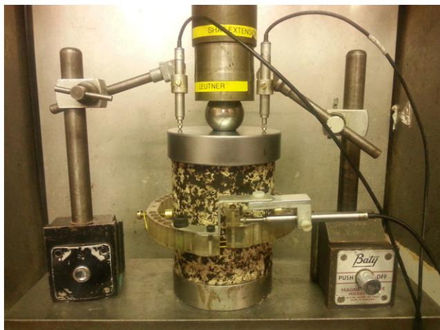
Figure 1. Test set-up for uniaxial indirect tension test
