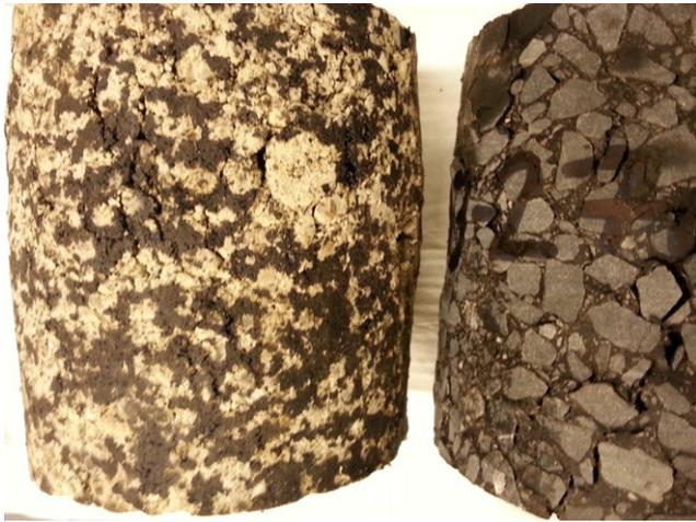
Figure 2. Foamed bituminous mixture and DBM90 samples after testing
