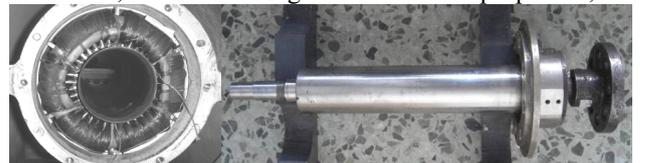
Fig. 3. Prototype stator and rotor.
