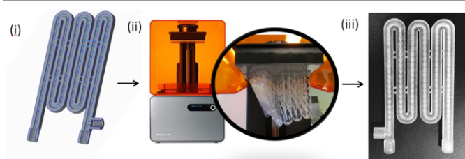
Figure 1: The stages of AM fabrication of a mini-OBR device. (i) A CAD model was designed to meet requirements. (ii) The reactor device was fabricated using Form2 SLA printer. (iii) The reactor was polished, cleaned and extensively flushed with IPA to remove residual uncured resin.
