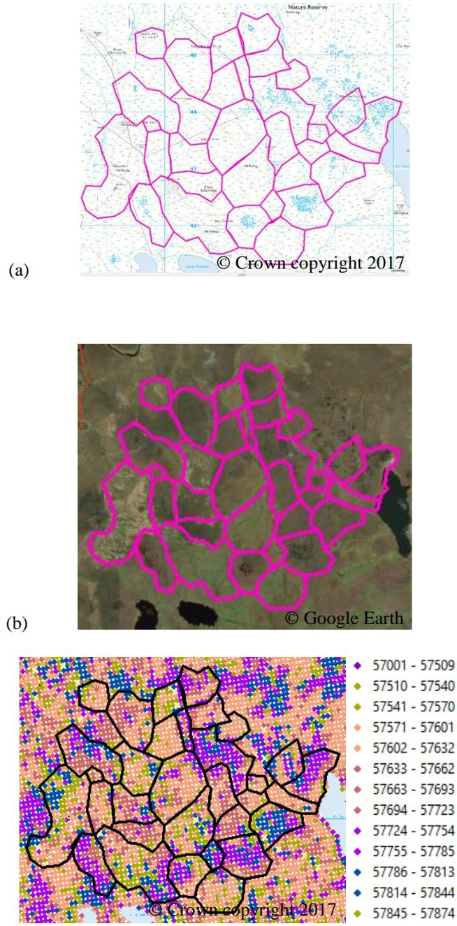
**Fig. S2.** Example of polygon definition using topographic context, clues to management and vegetation contrasts from, (a) UK Ordnance Survey map (Digimap Licence) © Crown copyright 2017. Distributed under the Open Government Licence (OGL). (b) True colour image, © Google Earth, and (c) Peak timing for 2016-2017 (key: serial date from 01/01/1901), for sub-site 3 Munsary.
