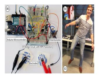
Figure 1. (a) GVS circuit used in the study; (b) electrode placement behind player's ears; (c) a player smiles as he feels his balance being affected.
