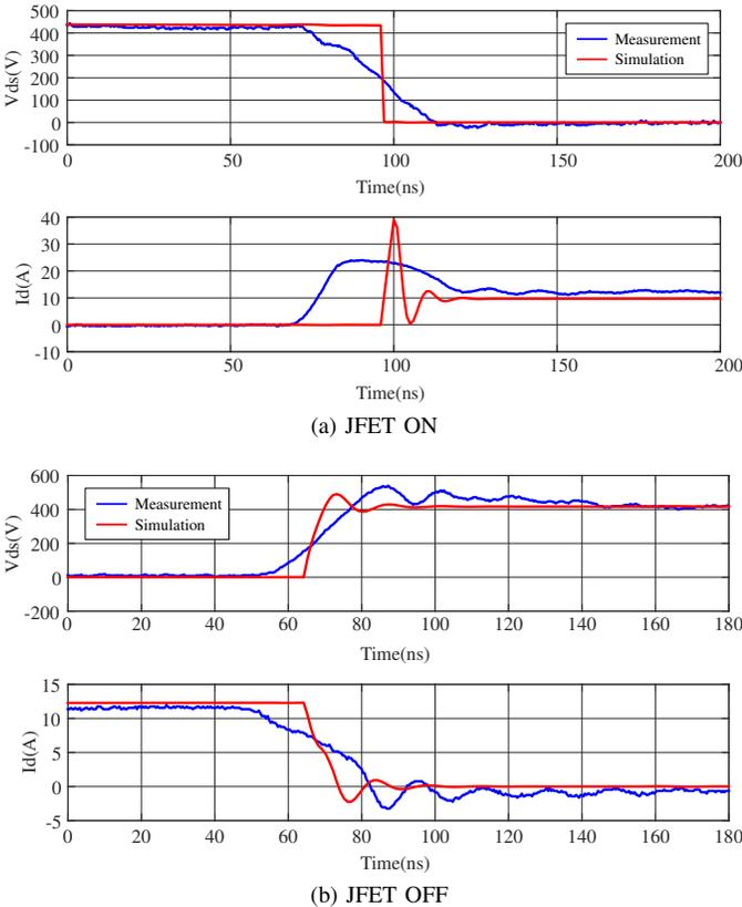
Fig. 8: JFET switching waveforms comparison of condition 1
