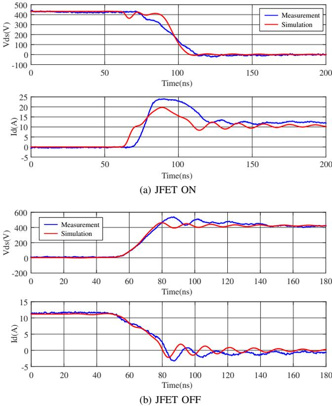
Fig. 10: JFET switching waveforms comparison of condition 3
