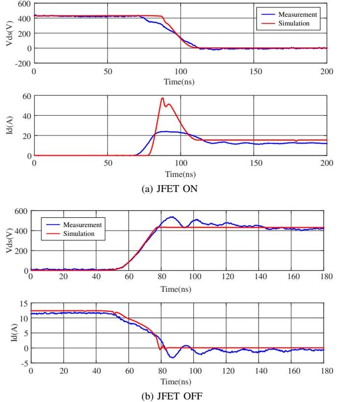
Fig. 9: JFET switching waveforms comparison of condition 2
