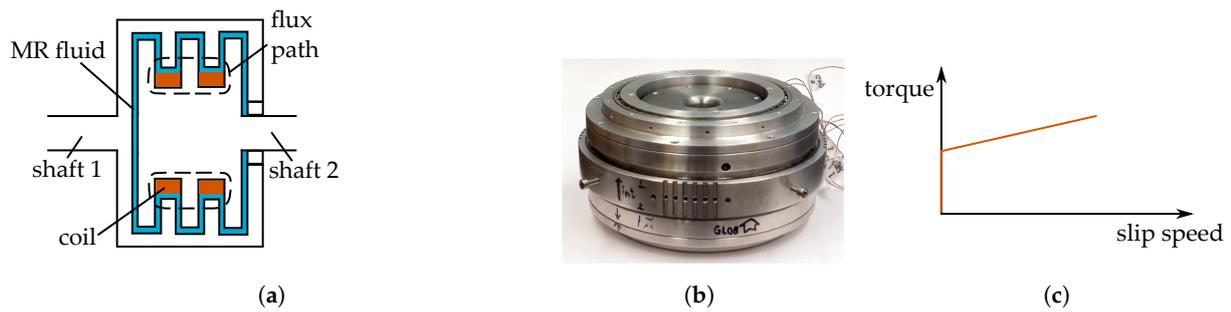
**Figure 9.** Of magneto-rheological (MR) fluid clutch: (a) Illustration (b) Photograph of a MR-fluid clutch for robotic application [39] (c) Torque vs. slip speed characteristics.
