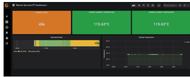
(a) Visualisation service for the Warren Services pilot study using Grafana engine.
