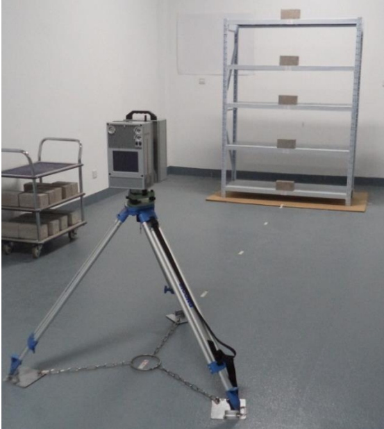
Fig. 3a: Scanning using the HDS7000 scanner
