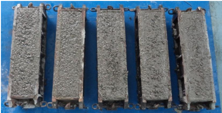
Fig. 1: Concrete specimens cast in steel moulds
