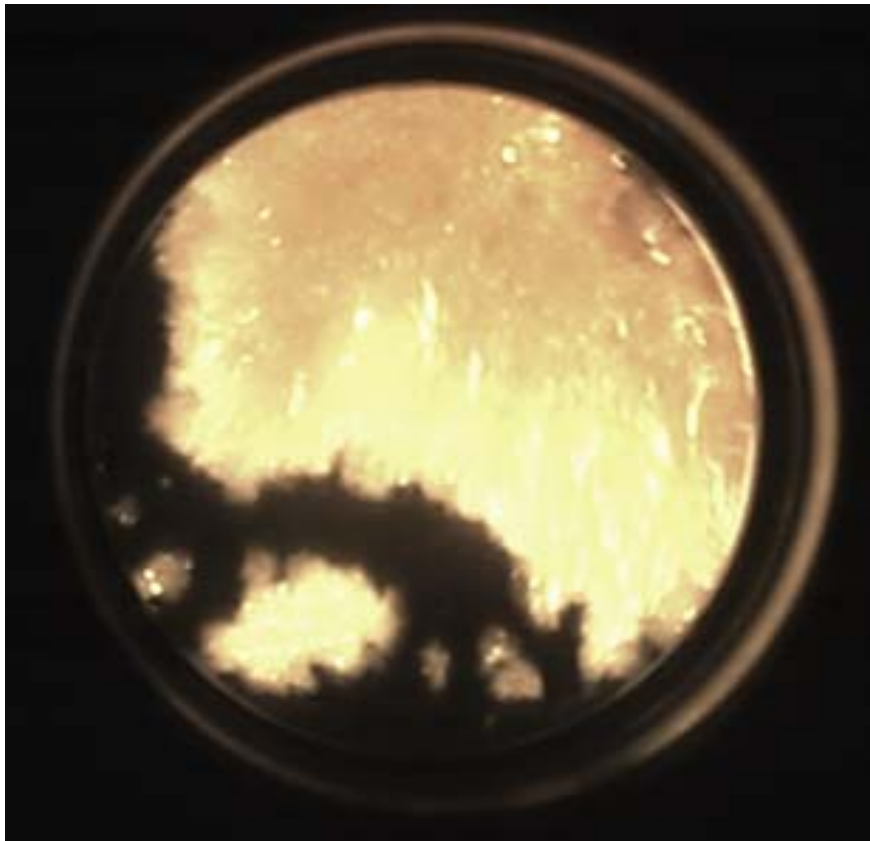
Figure 13: Blown-up intensified view of the multiple auto-ignition initiation sites observed during the baseline heavy knock cycle shown in Figure 10
