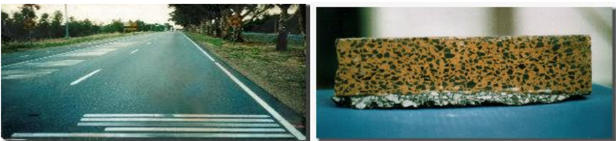
21 22 23 24 25 26 Figure 4: On the left, biobinder test road section near Adelaide, Australia. On the right, the Eco-pave™ 27 biobinder cross-section specimen [78, 79].
