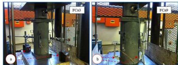
Fig. 5 (a) Horizontal potentiometers fixed on the base (b) Horizontal potentiometers fixed on the specimen.
