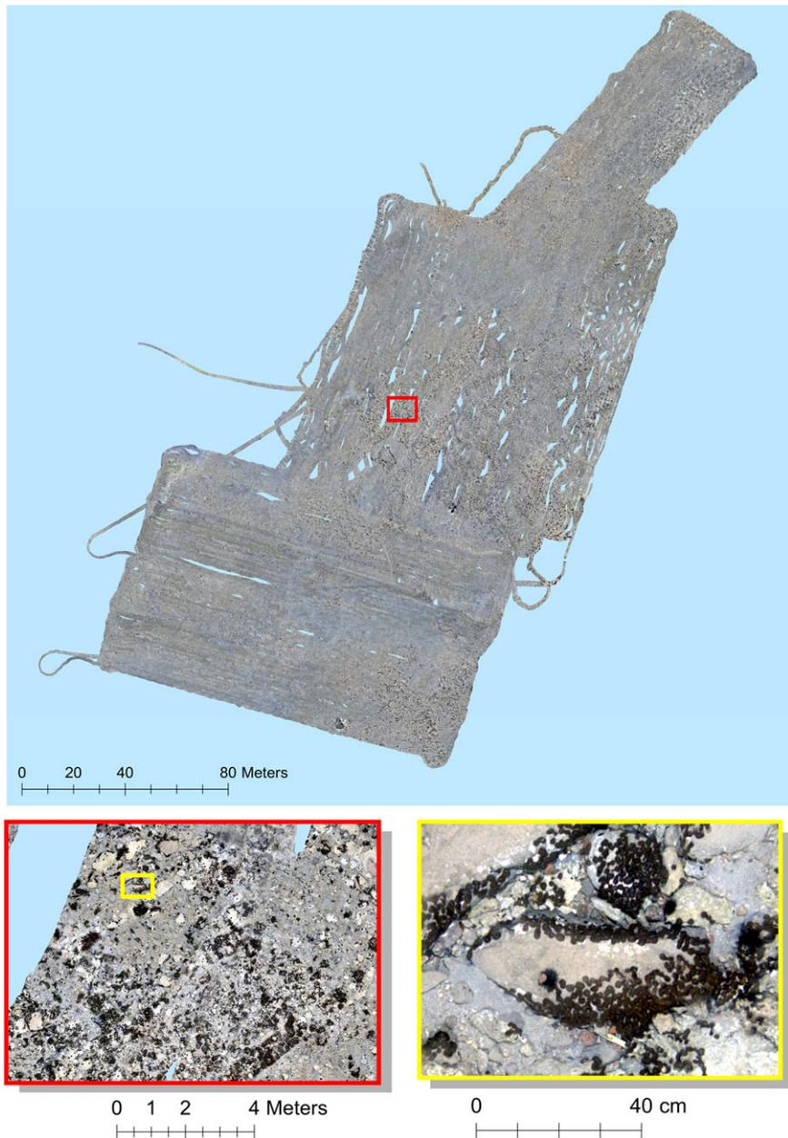
**Figure 17.** 3D model from the 2011 field season. This model is the result of a bundle adjustment of approximately 400,000 Iver2 gathered images into a large scale 3D model in which individual stones can be seen and mapped across the entire site.
