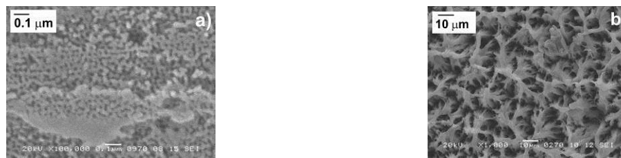
Figure 5: SEM images of the external surface of the sample obtained in sulphuric acid, the electrolysis time 4 h (a) and 6 h (b).
