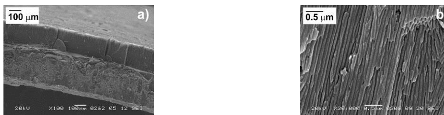
Figure 3: SEM images of the cross-cut section of the AAO layers prepared in oxalic acid: a) magnitude 100, b) magnitude 30000.
