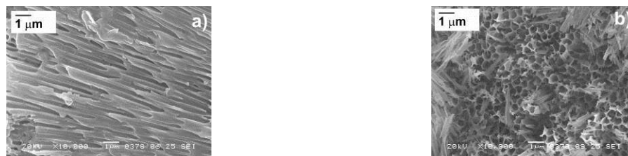
Figure 6: SEM images of the cross-cut section of the layers prepared in phosphoric acid, a) the cross-cut end, b) the external surface.
