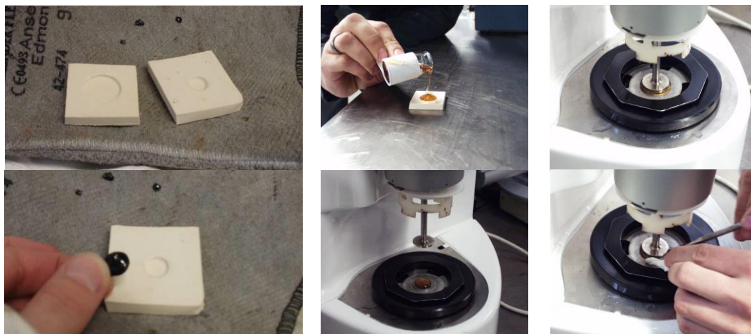
Figure 1. Methodology for preparing and loading polyacrylate binders and blends into the DSR: 25 mm and 8 mm silicone moulds and binder samples; pouring and placing binder samples in DSR; and setting final testing gap and trimming excess binder around testing geometry
