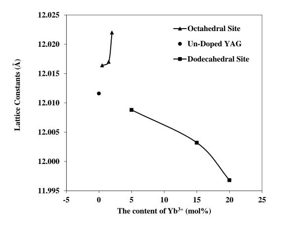
Figure 11: The change of lattice constant with Yb<sup>3+</sup> doping concentration in YAG.
