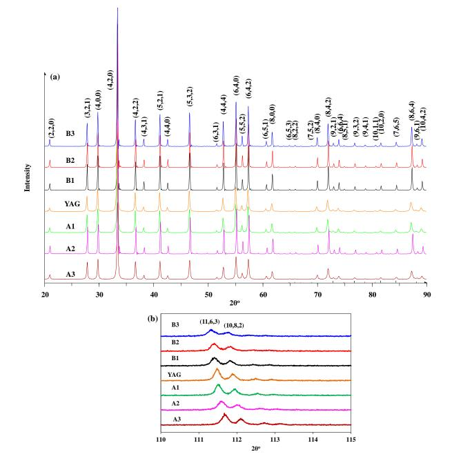
Figure 9: XRD patterns of Yb<sup>3+</sup> ions doped on dodecahedral and octahedral sites in YAG and undoped YAG powders (**a**)  $2\theta$  from 20 to  $90^{\circ}$ ; (**b**)  $2\theta$  from 110 to  $115^{\circ}$ .
