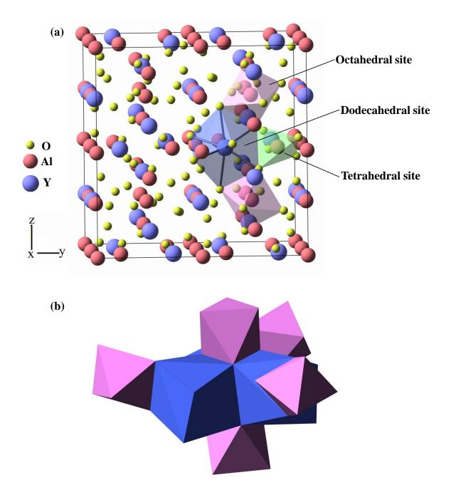
Figure 8: (a) The crystal structure of Yttrium aluminium garnet, in which there are three polyhedrons: dodecahedron, octahedron and tetrahedron; (b) one octahedron sharing its three edges with three different shared-edge dodecahedrons.
