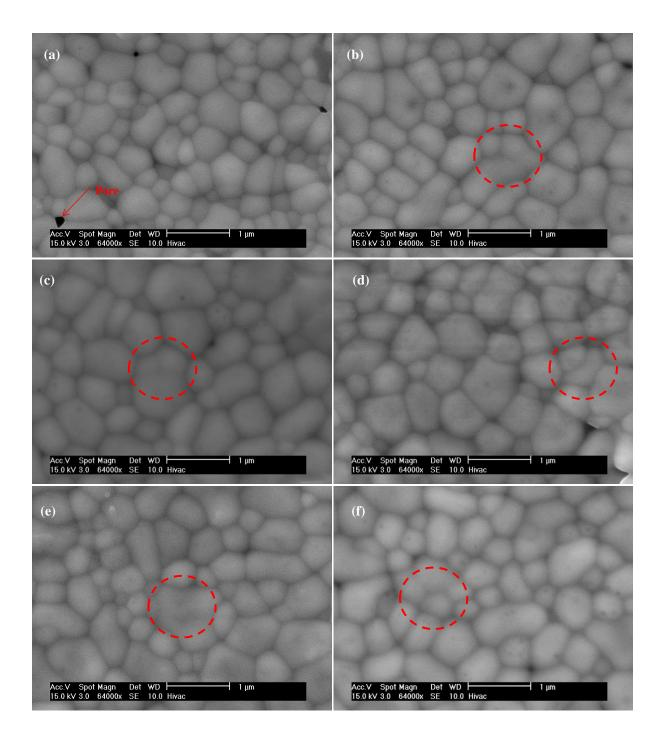
Figure 12: SEM images of the pellet surface: (a)  $(Yb_{0.05}Y_{0.95})_3Al_2Al_3O_{12}$ , A1; (b)  $(Yb_{0.15}Y_{0.85})_3Al_2Al_3O_{12}$ , A2; (c)  $(Yb_{0.2}Y_{0.8})_3Al_2Al_3O_{12}$ , A3; (d)  $Y_3(Yb_{0.005}Al_{0.095})_2Al_3O_{12}$ , B1; (e)  $Y_3(Yb_{0.015}Al_{0.085})_2Al_3O_{12}$ , B2; and (f)  $Y_3(Yb_{0.02}Al_{0.08})_2Al_3O_{12}$ , B3. Where the red circles regions present the recrystallization
