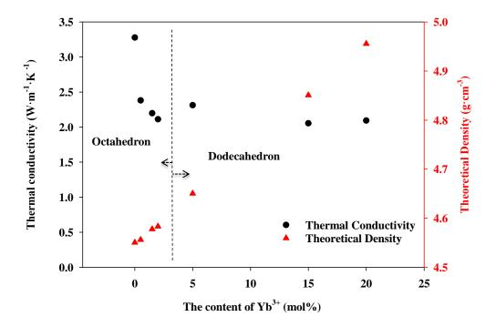
Figure 13: Thermal conductivities and theoretical densities of Yb<sup>3+</sup> ions doped YAG in dodecahedron or octahedron and un-doped YAG at room temperature.
