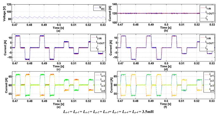
Fig. 6. Simulation results with balanced inductances: (a) DC-Link voltage; (b) Current HB 1; (c) Current HB 2; (d) Current HB 3; (e) X-axis leg currents; (f) Y-axis leg currents.
