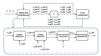
Fig. 5. Independent leg predictive current control block diagram.
