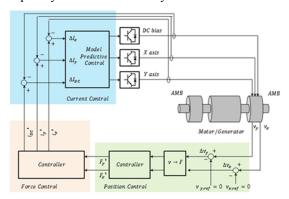
Fig. 4. Overall AMB system control scheme.
