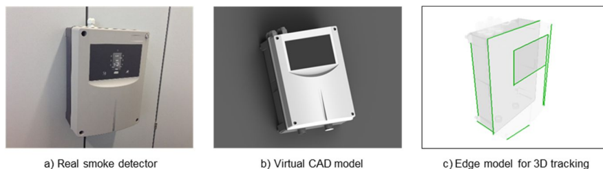
Figure 1: Demonstration object to verify the hybrid 3D tracking
