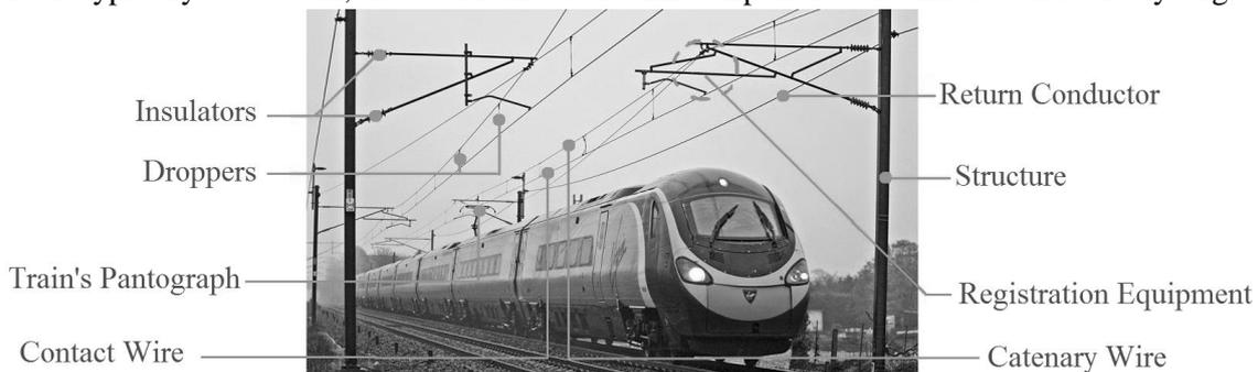
Figure 1. The Main OLE Components
