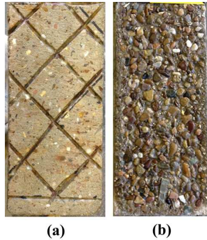
Fig. 3 Different concrete surface preparation: (a) grinding and creating a grid of grooves; and (b) sandblasting
