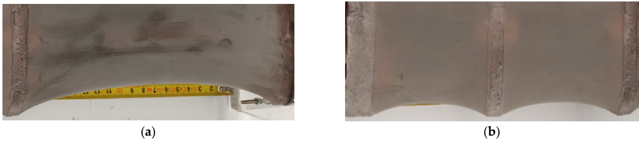
Figure 22. Poisson's contraction in latex skin at 25% span extension: (a) Without riblet. (b) With riblet.
