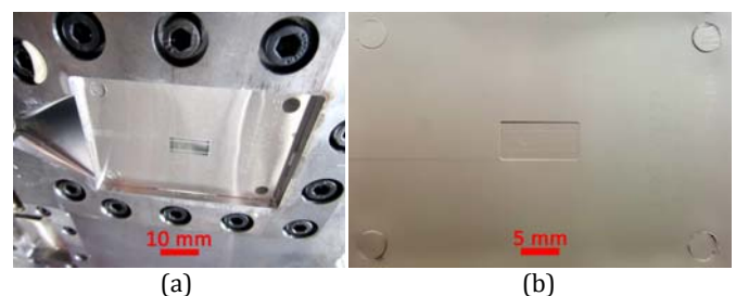
Figure 1. (a) Example of Rubert's nickel transfer standards used as mould insert; (b) example of polymer replica.
