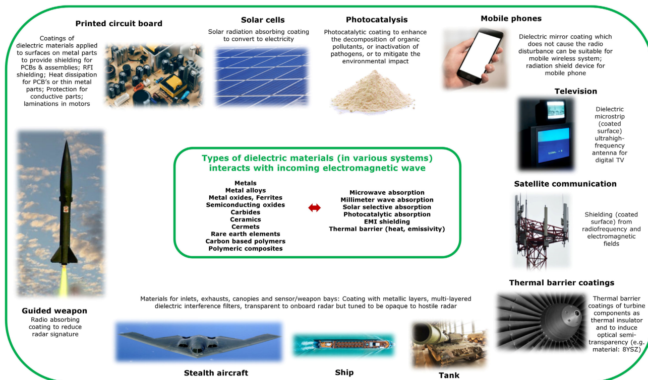
Figure 1. Example applications of dielectric material that can interact with EM waves and how their manufacturing using coating techniques can address the technological requirements.
