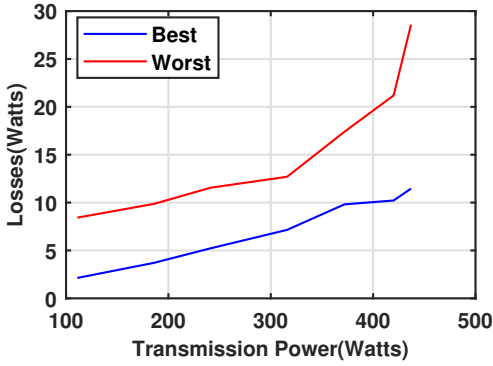
Fig. 11. Transformer losses in best and worst modes with Input Voltage V_1 = 230V , Output Voltage V_2^{ref} = 138V , Conversion ratio d=0.6 and switching frequency f=20kHz .
