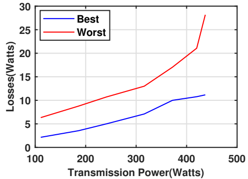
Fig. 15. Transformer losses in best and Worst modes(Experimental) with Input Voltage V_1 = 230V , Output Voltage V_2^{ref} = 138V , Conversion ratio d=0.6 and switching frequency f=20kHz .
