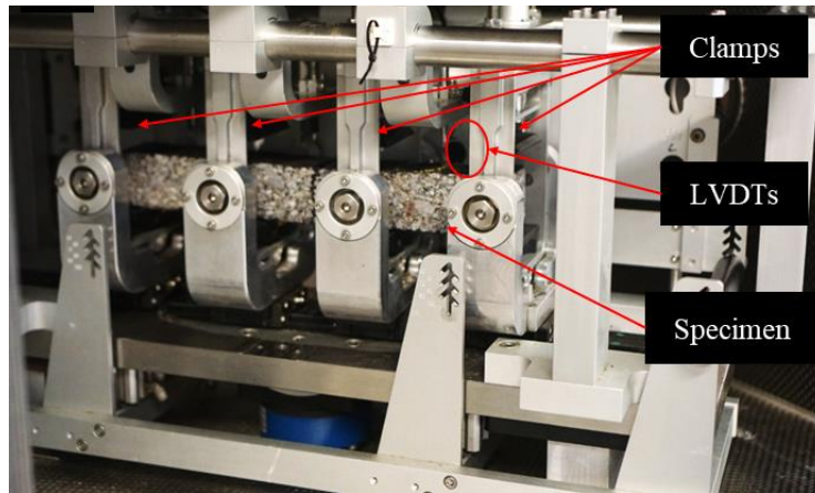
Figure 4: Setup and sketch of 4PB test.
