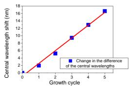
Figure S3: ZIF-8 deposition onto the surface of LPG with period of 110.7  $\mu m$ , central wavelength shift as a function of growth cycle
