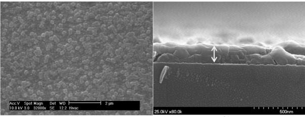
Figure 4: a) Top view and b) cross sectional SEM images of ZIF-8 films grown on glass substrates with 5 and 10 growth cycles respectively
