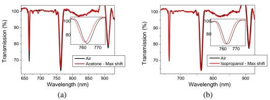
Figure S4: Transmission spectra of the LPG sensor with 5 growth cycles of ZIF-8 film exhibited to a) acetone and b) 2-propanol
