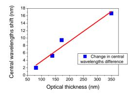
Figure 9: The change in the separation of central wavelengths corresponding to  $LP_{019}$  cladding mode induced by the deposition of ZIF-8 as a function of optical thickness
