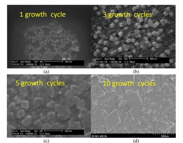
Figure S1: SEM images of ZIF-8 film comprised of a) one, b) three, c) five and d) ten growth cycles (the white at the bottom corresponds to 500 nm)
