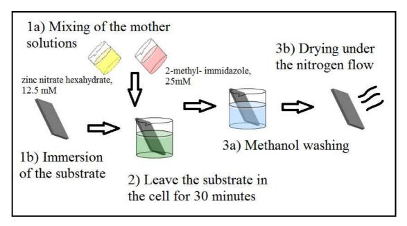
Figure 2: ZIF-8 fabrication methodology [12]
