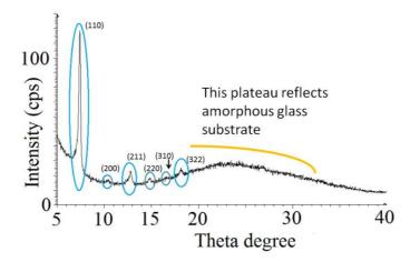
Figure 6: In-plane X-Ray diffraction patterns of ZIF-8 film grown on glass substrate via 20 growth cycles, recorded at room temperature
