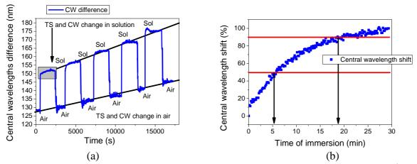
Figure 10: The dynamic shift of the central wavelength during the deposition of 1<sup>st</sup> to 5<sup>th</sup> growth cycle onto a surface of LPG and b) relative shift of the central wavelength during the immersion in the film forming solution over the deposition of 1<sup>st</sup> growth cycle
