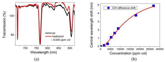
Figure 12: LPG sensor with 5 growth cycles of ZIF-8: a) shift in transmission spectrum corresponding to approximately 9,000 ppm of methanol and b) methanol calibration curve
