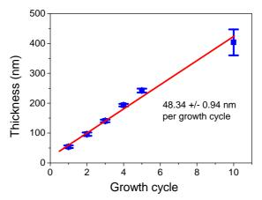
Figure 5: Ellipsometry measurement: thickness of ZIF-8 film as a function of growth cycle (average value is shown and error bars were calculated as the standard deviation from the measurement over the 3 substrates)
