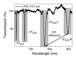
Figure 7: Transmission spectrum of the bare LPG with period of  $110.7\mu$ m measured in air with attenuation bands (grey frames) corresponding to the LP<sub>018</sub> and LP<sub>019</sub> cladding modes (the dual resonance was observed for the LP<sub>019</sub> cladding mode).
