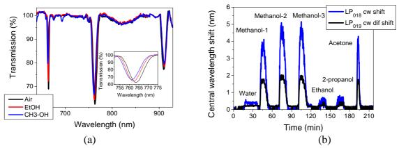
Figure 11: Transmission spectra of the LPG sensor with 5 growth cycles of ZIF-8 film exposed to methanol (blue) and ethanol (red) and b) dynamic shift of the shift of the central wavelength corresponding to LP<sub>018</sub> cladding mode (black) and the shift in the difference of the central wavelengths corresponding to LP<sub>019</sub> cladding mode (blue) of the LPG sensor coated with 2 growth cycles of ZIF-8 as the response to different organic vapours and water (for comparison)
