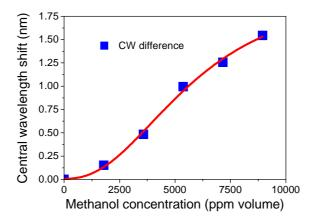
Figure S5: LPG sensor coated with 2 growth cycles of ZIF-8 - Methanol calibration curve
