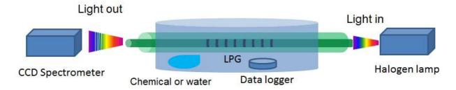
Figure 3: Experimental set-up for chemical sensitivity experiments.
