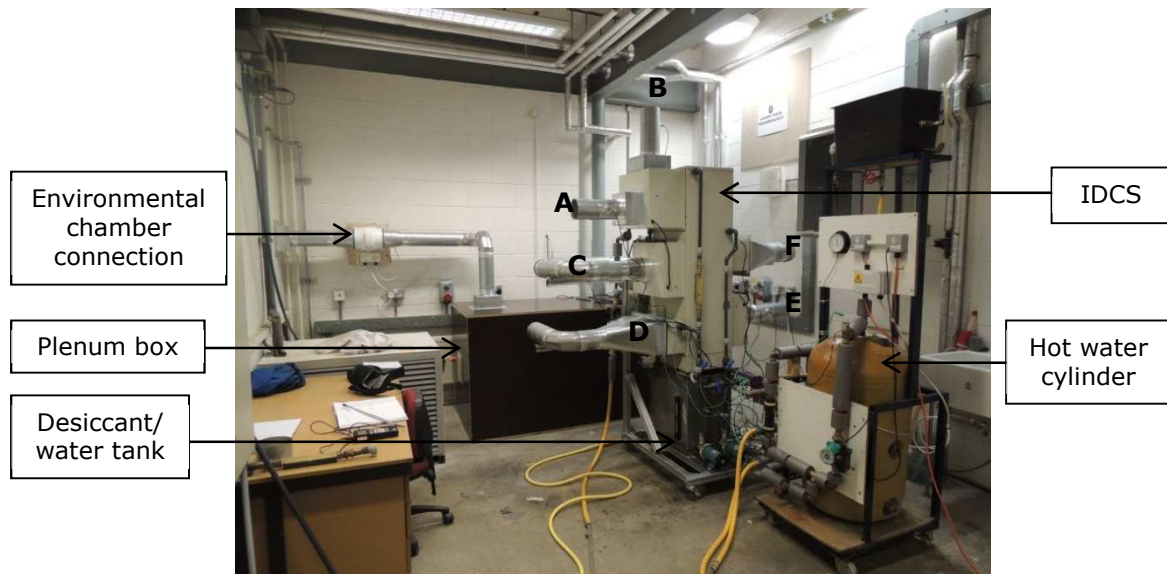
Figure 5 IDCS laboratory setup with labelled air flows
