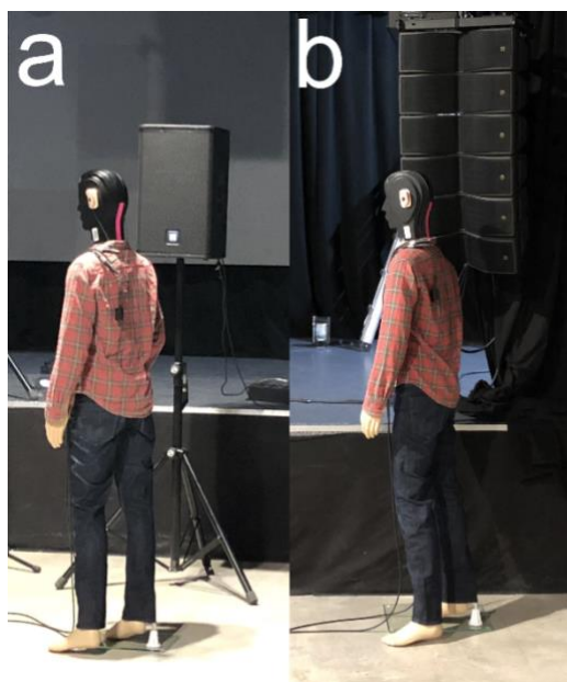
Figure 2 Photographs of the dummy head and mannequin in front of (a) the point-source loudspeaker and (b) the line-array system.
