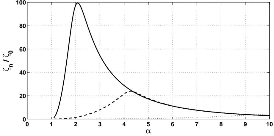
Figure 3: The impact of  $\eta$  on the damping ratio enhancement  $\zeta_n/\zeta_0$  of the suggested oscillator with  $m_2=0$ :  $\zeta_0=0.1$  ( $\cdots$ ),  $\zeta_0=0.01$  ( $-$ ),  $\zeta_0=0.001$  ( $-$ ). All computations conducted with  $\varepsilon=5\%$ .
