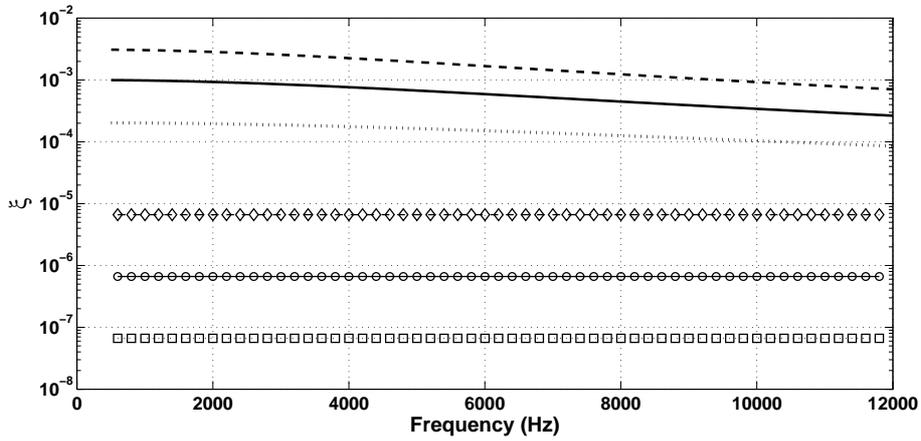
Figure 8: Damping ratio  $\xi$  as a function of frequency for the flexural wave propagating within the beam. Results for the SDoF oscillator:  $\eta=0.01$  ( $\square$ ),  $\eta=0.1$  ( $\circ$ ),  $\eta=1$  ( $\diamond$ ). Results for the mechanism having negative stiffness inclusions:  $\eta=0.01$  and  $\alpha=1.2$  ( $\cdots$ ),  $\eta=0.1$  and  $\alpha=1.6$  (—),  $\eta=1$  and  $\alpha=3$  (---).
