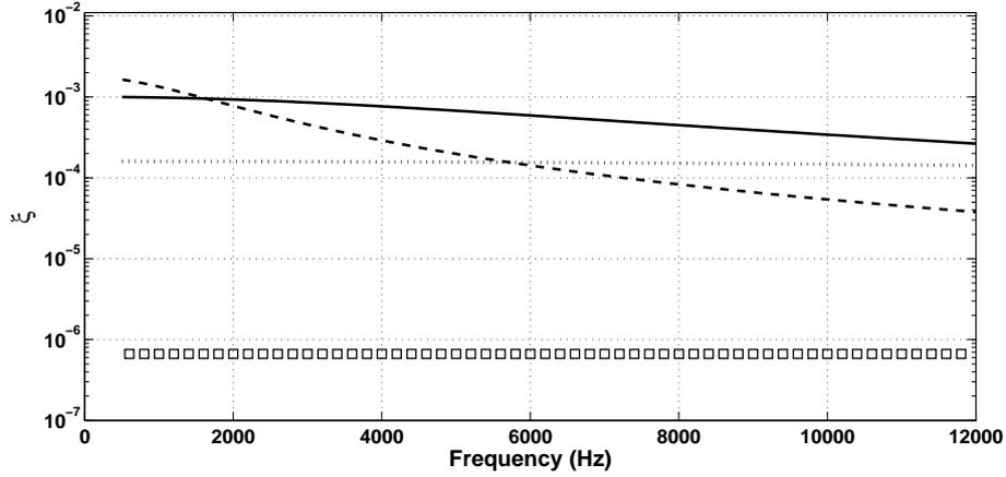
Figure 9: Damping ratio  $\xi$  as a function of frequency for the flexural wave propagating within the beam for  $\eta=0.1$ . Result for no negative stiffness ( $\square$ ). Results for the mechanism having negative stiffness inclusions:  $\alpha=1.3$  (- -),  $\alpha=1.6$  (- · -),  $\alpha=2.5$  (· · ·).
