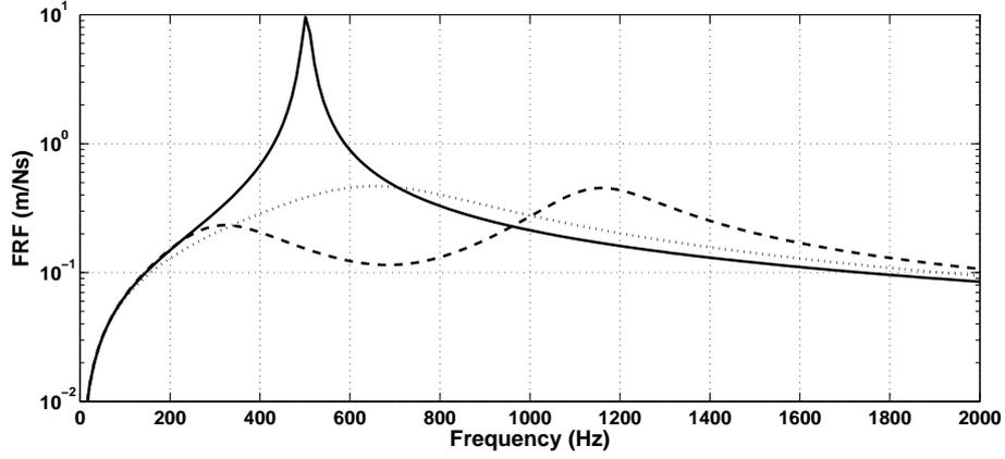
Figure 2: Comparison of the FRF  $V_x/F$  for: the SDOF system (—), the modified oscillator with  $m_2=0$  (···) and the modified oscillator with  $m_2=0.05m_1$  (- -). The design parameters of the system are  $\varepsilon=5\%$  and  $\alpha=3.3$  while  $\eta=10\%$ .
