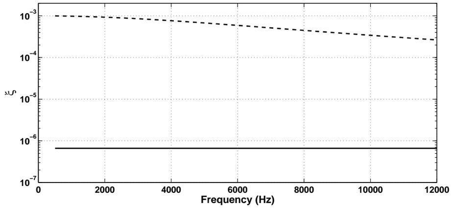
Figure 7: Damping ratio  $\xi$  as a function of frequency for the flexural wave propagating within the beam: No negative stiffness (—), With negative stiffness inclusions (---). Computations conducted with  $\alpha=1.6$ ,  $\eta=0.1$
