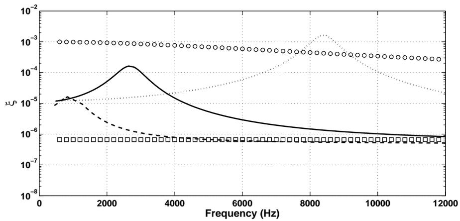
Figure 11: Damping ratio  $\xi$  as a function of frequency for the waves propagating within the beam for  $\eta=0.1$ . Result for no negative stiffness ( $\square$ ) and modified configuration with  $m_2=0$  ( $\circ$ ). Results for:  $m_2=0.3M$  (---),  $m_2=0.03M$  (-·-),  $m_2=0.003M$  (···).
