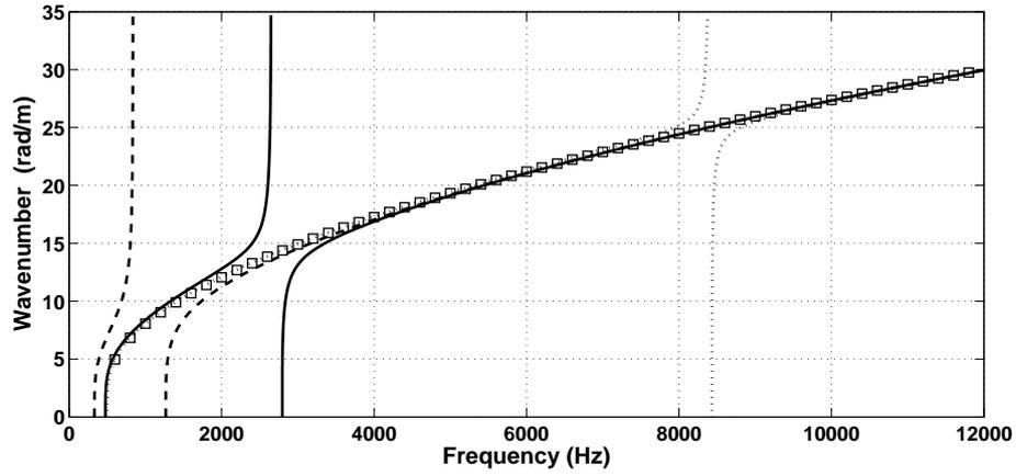
Figure 10: Wavenumber  $k$  as a function of frequency for the waves propagating within the beam. Result for no negative stiffness inclusions ( $\square$ ). Results for various values of  $m_2$ :  $m_2=0.3M$  (---),  $m_2=0.03M$  (-·-),  $m_2=0.003M$  (···). Computations conducted with  $\alpha=3$ ,  $\eta=0.1$
