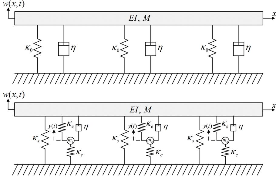
Figure 4: Illustration of an infinitesimal part of the considered beam. Top: The beam connected to the floor through a stiffness  $\kappa_0$  and a damping coefficient  $\eta$ . Bottom: The beam connected to the floor using the suggested mechanism with  $\eta$  equal to the precedent case,  $\kappa_s$ ,  $\kappa_e$  positive stiffness and  $\kappa_c$  negative stiffness elements.
