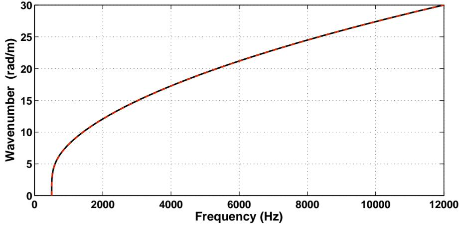
Figure 6: Wavenumber  $k$  as a function of frequency for the flexural wave propagating within the beam: No negative stiffness (—), With negative stiffness inclusions (---). Computations conducted with  $\alpha=1.6$ ,  $\eta=0.1$
