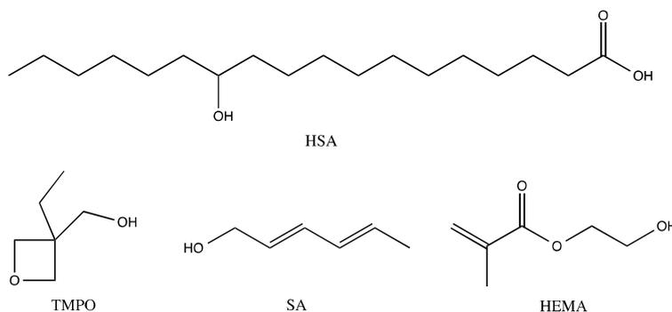
**Figure 2 - The functional end-cappers used in this study.**
