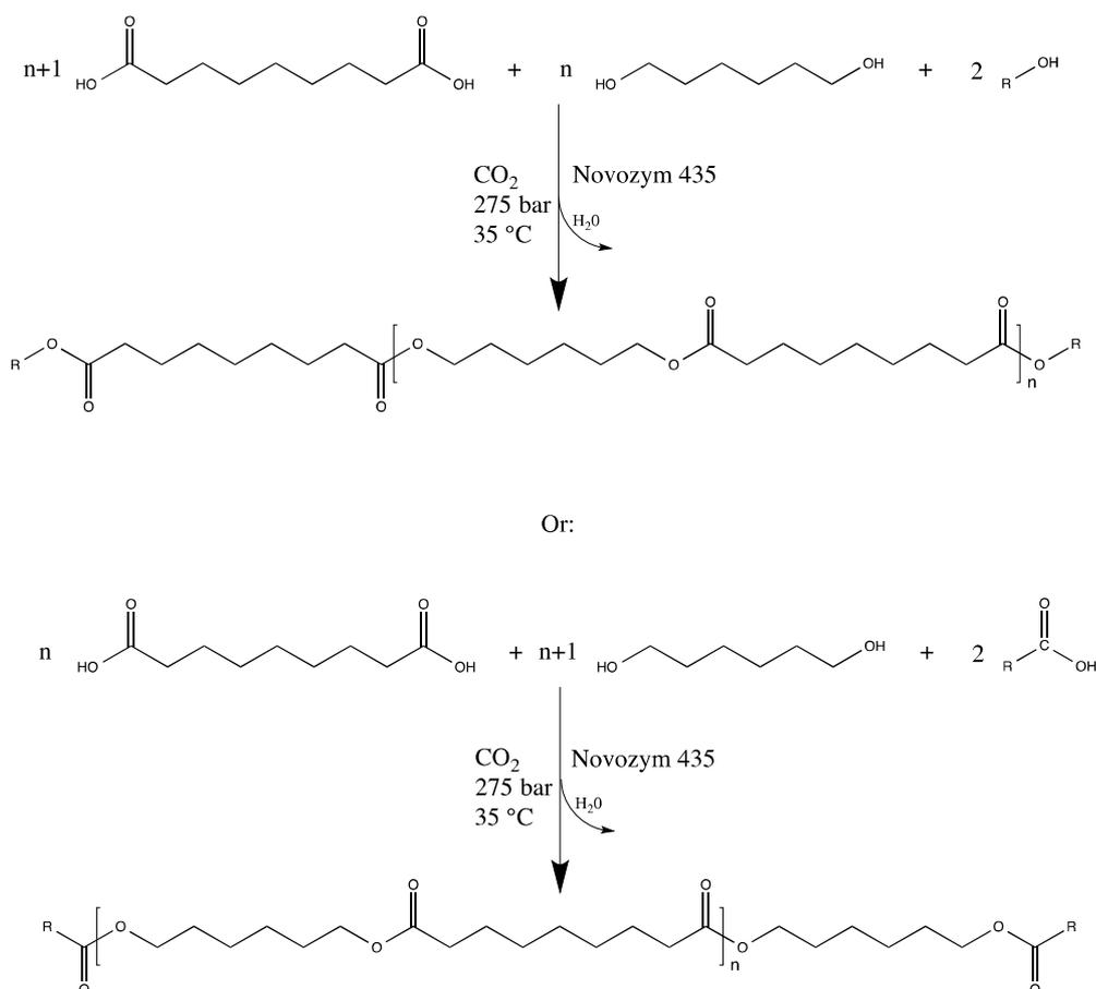
**Figure 3 – Reaction schemes for the enzymatic syntheses of the green telechelics in  $s\text{CO}_2$ . An excess of diacid was used for alcohol end-cappers (SA, HEMA and TMPO), whilst an excess of diol was required in the case of the acid end-capper (HSA).**
