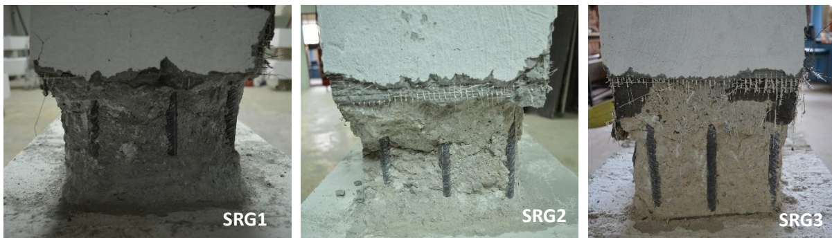
Fig. 15: State of the core cross section in the critical region after removal of the textile.
