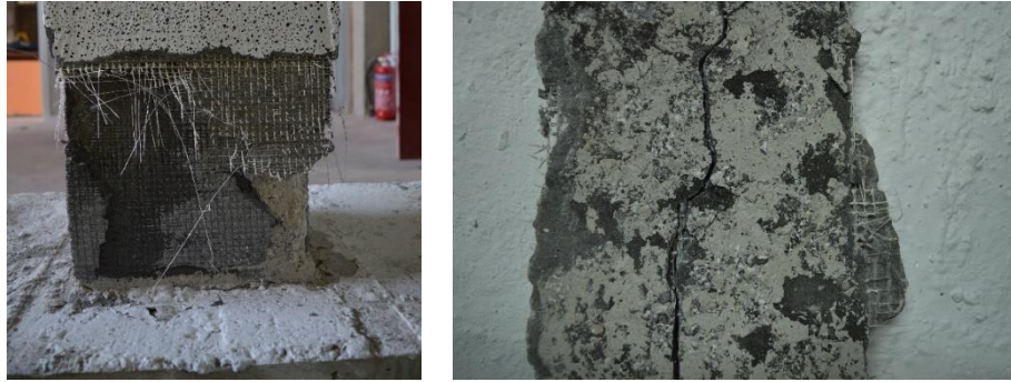
Fig. 16: State of the critical region after the removal of the textile.
