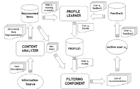
Fig. 1. High level architecture of a Content-based recommender system
