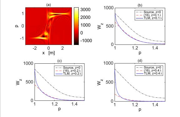
**Figure 8.** (a) Source distribution; near-field  $\Re \{W_z\}$  WDF: comparison between TLM computation and evanescent-wave approximation (16) for (b)  $z = 0.1\lambda$ ; (c)  $z = 0.2\lambda$  and (d)  $z = 0.4\lambda$  along x = 0. The range of p at x = 0 is restricted between 1 and 1.5 in (b)–(d) in order to emphasize the behavior of evanescent waves in phase-space.
