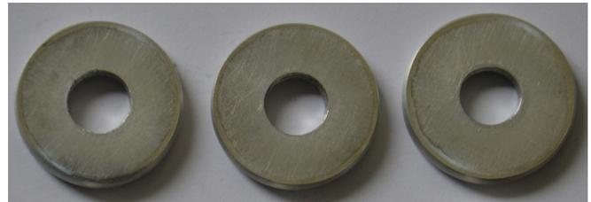
Fig. 15. The ring workpiece after compression under the dry dies.
