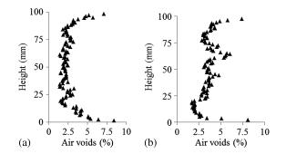
Fig. 5. Specimen A: air void distribution for (a) V-mix; (b) RA30-mix
