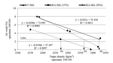
**Fig. 8.** Relationships of the target air void content for 100/100 specimen and the density to be set during compaction for 150/150 specimen
