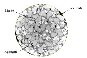
Fig. 3. 2D X-ray CT image of the specimen
