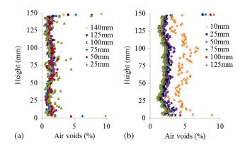
Fig. 7. Specimen C: inner cores (a) and outer rings; (b) analyses of compacted RA30-mix specimen
