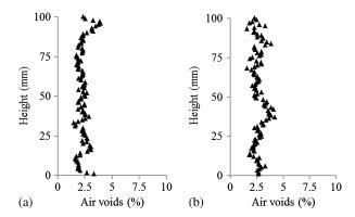
**Fig. 9.** Specimen C  $(100 \times 100 \text{ mm core})$ : air void distribution for (a) V-mix; (b) RA30-mix
