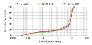
Fig. 1. Aggregate grading curves of V-mix and RA-mixes
